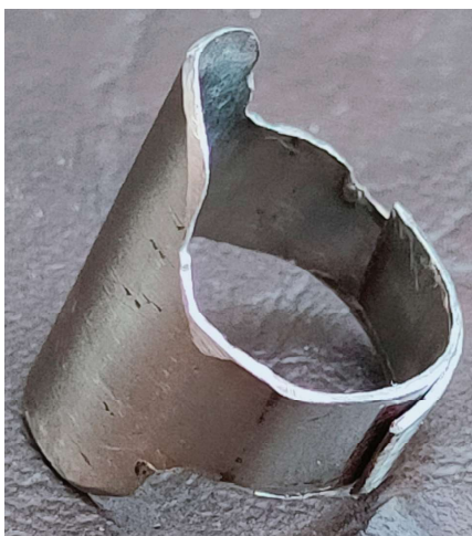
Fig. 3.4.1 Finger tool for peeling cashew
