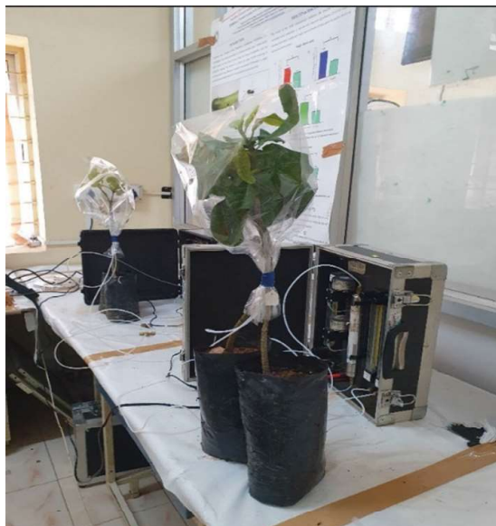
Fig. 3.3.6 Set up for collectin of plant volatiles and conducting bioassys
