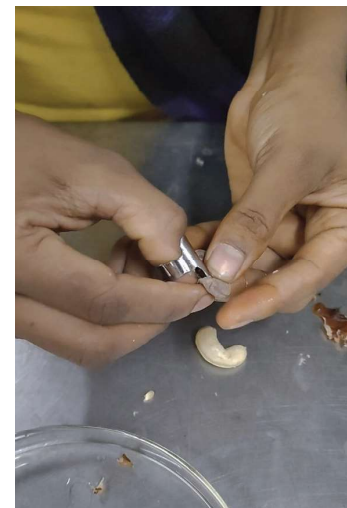
Fig.3.4.2 Manual peeling of unpeeled cashew using finger tool
