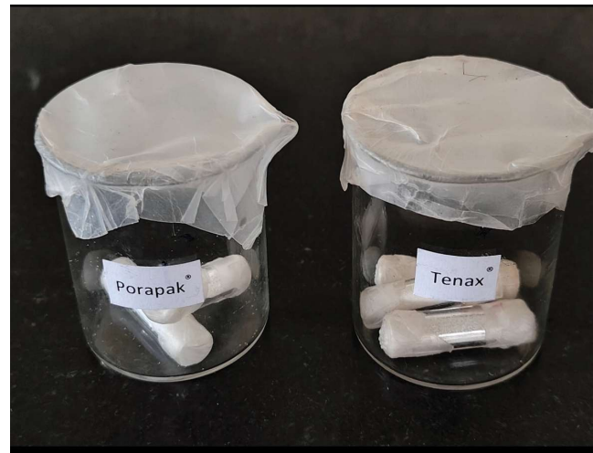
Fig. 3.3.1b Volatiles adsorbed onto Tenax® or Porapak® cartridges for future evaluation.
