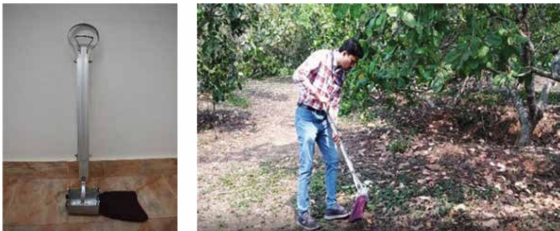
Fig. 3.2.19 A view of Jaw-type fruit collector
