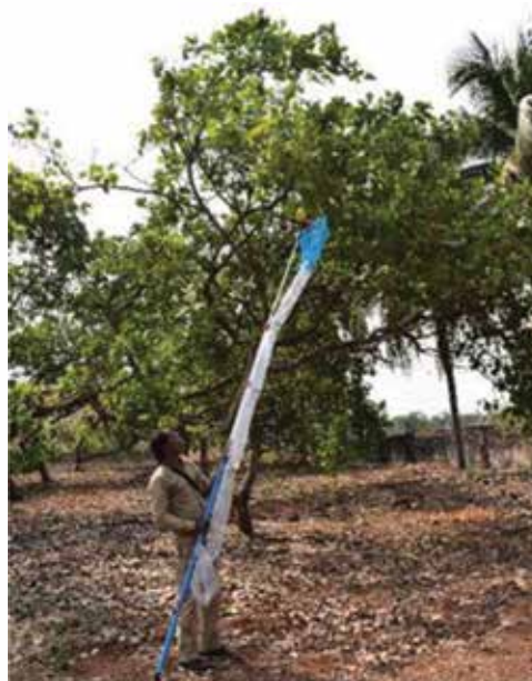
Fig. 3.2.17 A view of Battery-operated telescopic cashew fruit harvester
