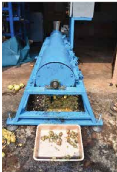
Fig. 3.2.16 A View of cashew fruit & nut separator in operation
