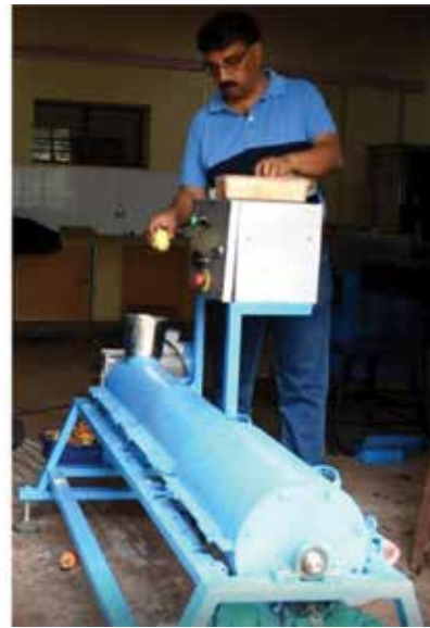
Fig. 3.2.16 A View of cashew fruit & nut separator in operation
