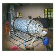
Size grading of raw cashewnuts prior to processing is the first step in mechanization. Graded cashewnuts reduces work load in subsequent process of shelling, peeling and grading to achieve the goal of
