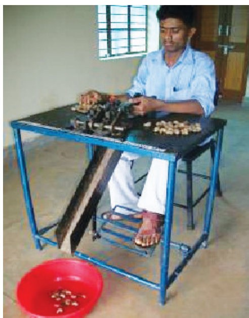
Fig. 4.9: Radial arm type cashew kernel extractor machine
